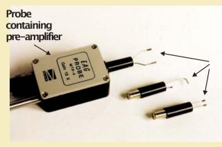
Interchangeable electode holders for different sizes of antennae
