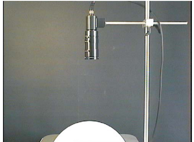
CMOS sensor and zoom lens
