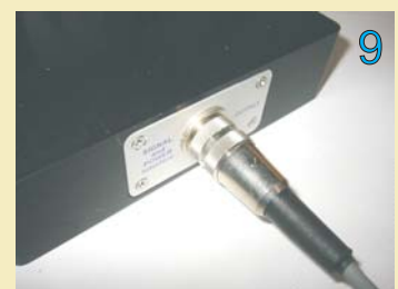
Signal/Power interface cable connection
