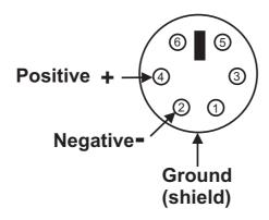
This is the INSIDE (solder side) of the mini DIN plug
